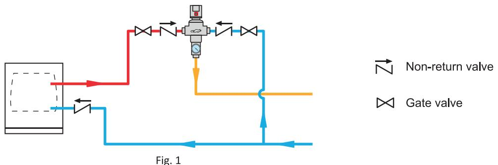
(EN) Installation diagram with recycling circuit
